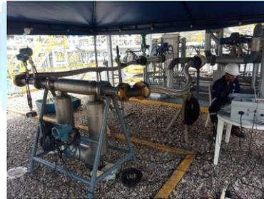
Este servicio se lleva a cabo de acuerdo a instrucciones de las normas ISO 10790:2015 Measurement of fluid flow in closed conduits — Guidance to the selection, installation and use of Coriolis flowmeters (mass flow, density and volume Flow measurements). Anexo A Y la ISO 5168:2005 Measurement of fluid flow — Procedures for the evaluation of uncertainties 2 edición. Anexo H
